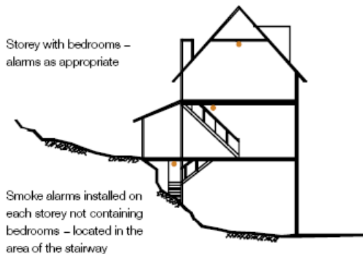
Diagram 4: Cross section through a dwelling showing smoke alarms in the storey containing bedrooms (top floor) and the storeys not containing bedrooms. Smoke alarms located within area of stairway
