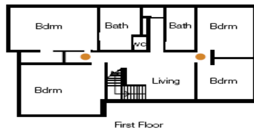
Diagram 3: Two storey dwelling showing smoke alarms in the storey containing bedrooms (first floor) and the storey not containing bedrooms (ground floor)
